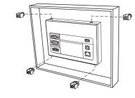
Tighten the screws with the torque less than 0.5 N-M / 0.7 N-M to avoid damage to the plastic clearance of 60 mm on the rear of the HMI. DOP-107PV torque: 6.17 lb-inch (0.7 N-M)
