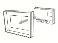
Tighten the screws with the torque less than 0.5 N-M / 0.7 N-M to avoid damage to the plastic
