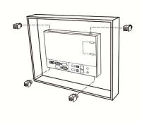
For heat dissipation, please keep a minimum clearance of 60 mm on the rear of the HMI.
