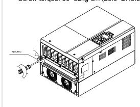
☑ Fasten 5 screws (as shown in the following figure). Screw torque: 30~32kg-cm (26.0~27.8lb-in).
