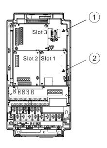
1 RJ45(Socket) for digital keypad
