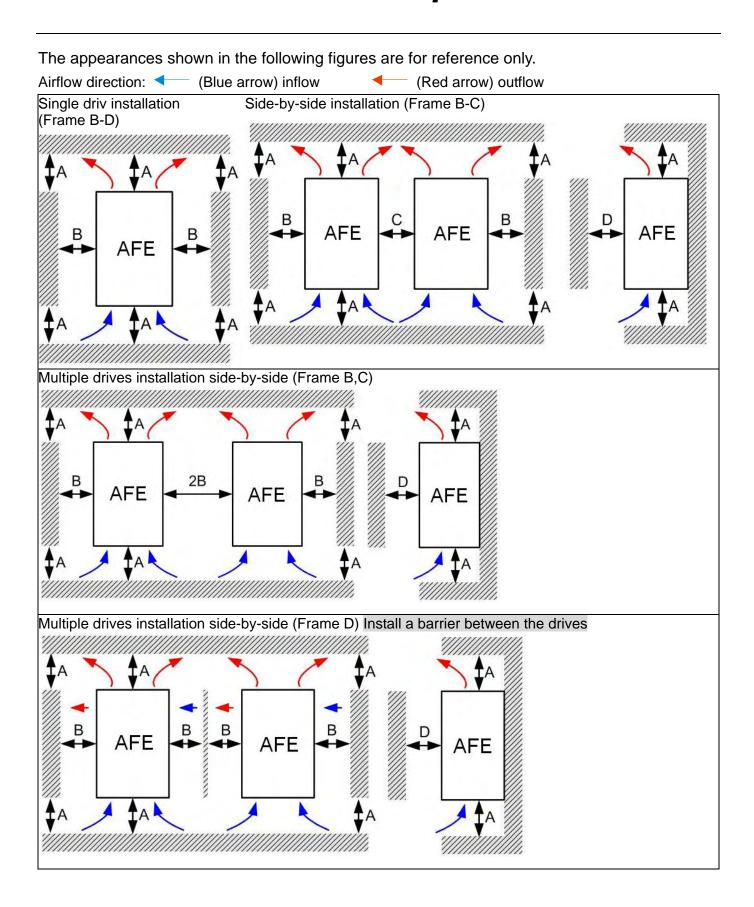
Multiple drives installation side-by-side in rows (Frame B,C) Ta: Frame B~D
