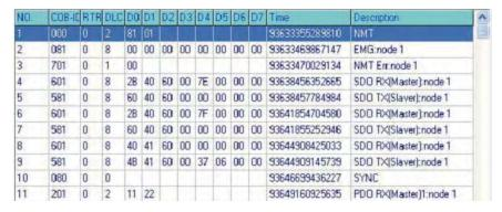
Master send NM message to slave 1 for RESET request. Slave 1 responds no error Slave 1 responds a boot up message Master enter Index6040 = 7EH in slave 1 Slave 1 responds OK Master enter Index6040= 7FH in slave 1 Slave 1 responds OK Master enter value for Index6041 to slave 1 Slave 1 responds 0640H Master enter SYNC
