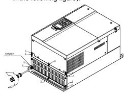
3. Fasten 4 screws (as shown in the following figure). 7. Screw torque: 30~32kg-cm (26.0~27.8lb-in).
