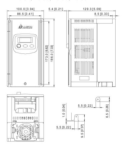
Frame S2: VFD015S21U, VFD015S43U, VFD022S21U, VFD022S43U
