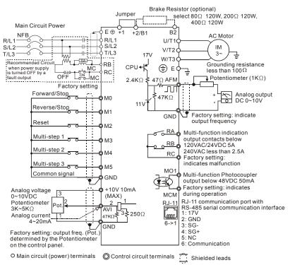
NOTE: Do not plug in a modem or telephone line to the RS-485 communication port, permanent damage may result. Pins 1&2 are the power sources for the optional copy keypad and should not be used while using RS-485 communication.
