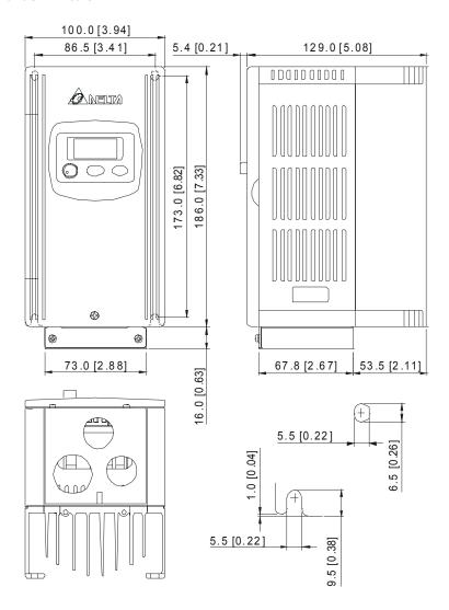
Frame S2: VFD015S21D, VFD015S21E, VFD015S43D, VFD015S43E, VFD022S21D, VFD022S21E, VFD022S23D, VFD022S43D, VFD022S43E
