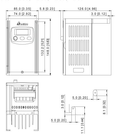
Frame S1: VFD004S43B, VFD007S43B
