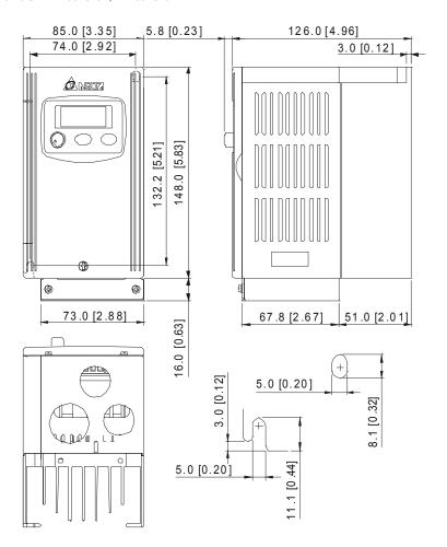
Frame S1: VFD002S21E, VFD004S21E, VFD007S21E, VFD015S23D
