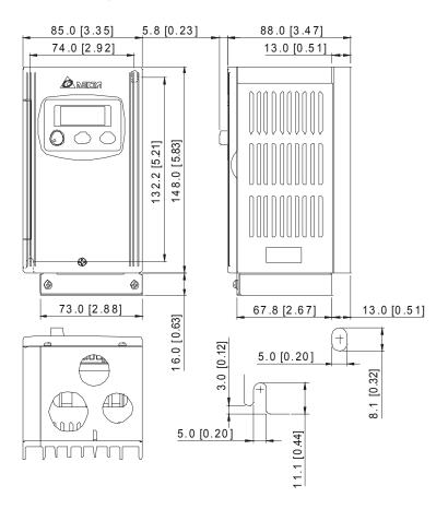
Frame S1: VFD004S11A, VFD004S21A, VFD004S23A
