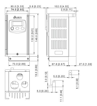
Frame S1: VFD007S21A, VFD007S23A
