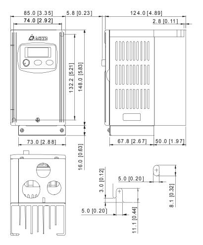
Frame S1: VFD004S43A, VFD004S43E, VFD007S43A, VFD007S43E
