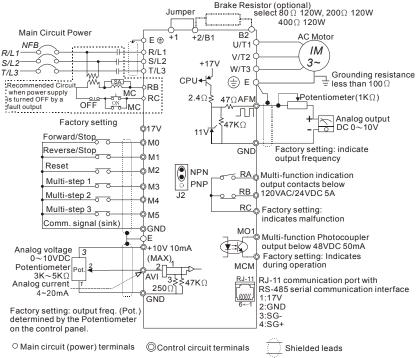
NOTE: Do not plug in a Modem or telephone line to the RS-485 communication port, permanent damage may result. Pins 1 & 2 are the power sources for the optional copy keypad and should not be used while using RS-485 communication.
