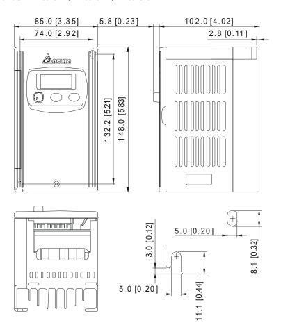
Frame \$1: VFD004S11B, VFD004S21B
