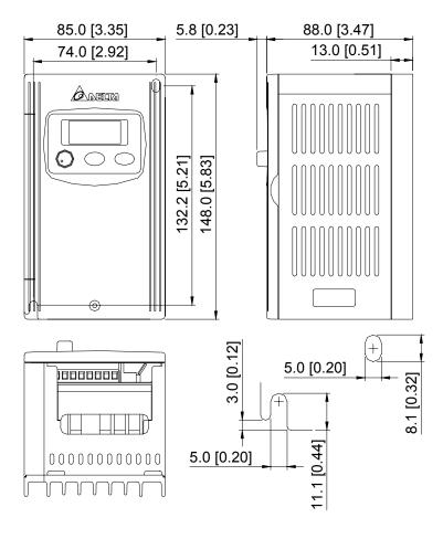
Frame S1: VFD002S11B, VFD002S21B
