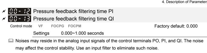
If the time constant is too large, a stable control is obtained with poorer control response. If it is too small, a fast response is obtained with unstable control. If the optimal setting is not known, adjust it
