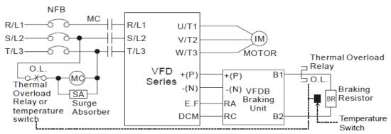
Note1: When using the AC drive with DC reactor, please refer to wiring diagram in the AC drive user manual for the wiring of terminal +(P) of Braking unit.
