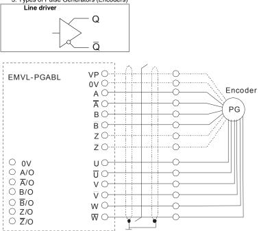
4. Output Signal Setting of the Frequency Divider
