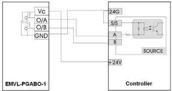
If the encoder type is line driver, when switch SW2 is set to +12V or +24V, the PG card will only output 5V.
