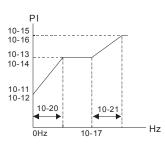
When using multi-function input terminals to switch ASR1/ASR2, the diagram will be shown as
