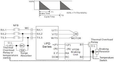
Note1: When using the AC drive with DC reactor, please refer to wiring diagram in the AC drive user manual for the wiring of terminal +(P) of Braking unit.
