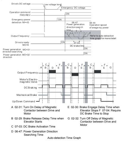
FOCPG/PM Control Mode: within the time setting of Pr.06-47, the drive maintains at zerospeed and it is able to determine the elevator loading without performing forward/reverse run. Then the elevator operates in power regeneration direction (the motor is in power generating status). Refer to the diagram below for the Auto-Detection Time Graph.
