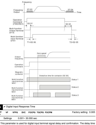
This parameter is used for digital input terminal signal delay and confirmation. The delay time is confirmation time to prevent some uncertain interferences that would result in error (except for the counter input) in the input of the digital terminals (FWD, REV and MI1~8). Under this condition, confirmation for this parameter could be improved effectively, but the response time will be somewhat delayed.
